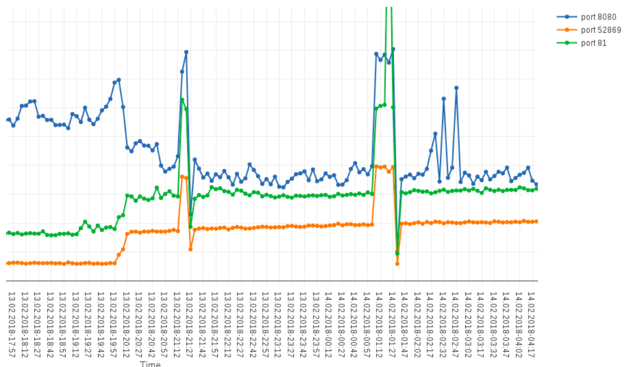
Figure 2.23: Satori change of tactics: scanning for vulnerable Huawei routers and IP cameras
